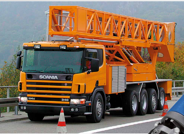
A WD-HC 0300 slew drive with multi-disk brake is located in the rotary boom linkage of this underbridge inspection device
